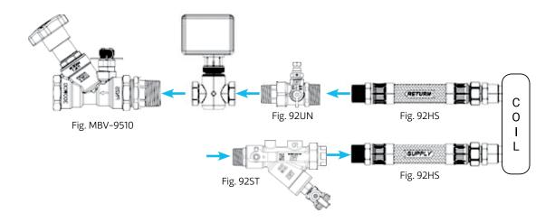
Multiple configurations available. Product will be seal packed and labeled per the mechanical schedule provided. For additional information on Gruvlok bag and tag coil kit service, contact an ASC Engineered Solutions Representative.
